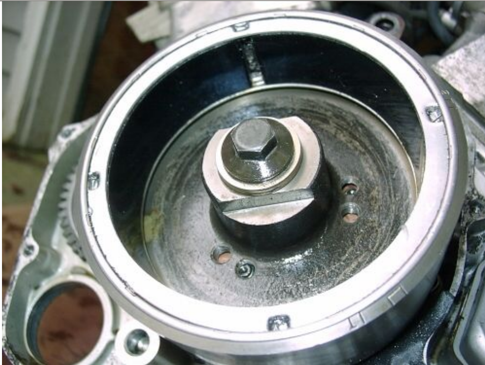
Flywheel with 2 magnets inside
