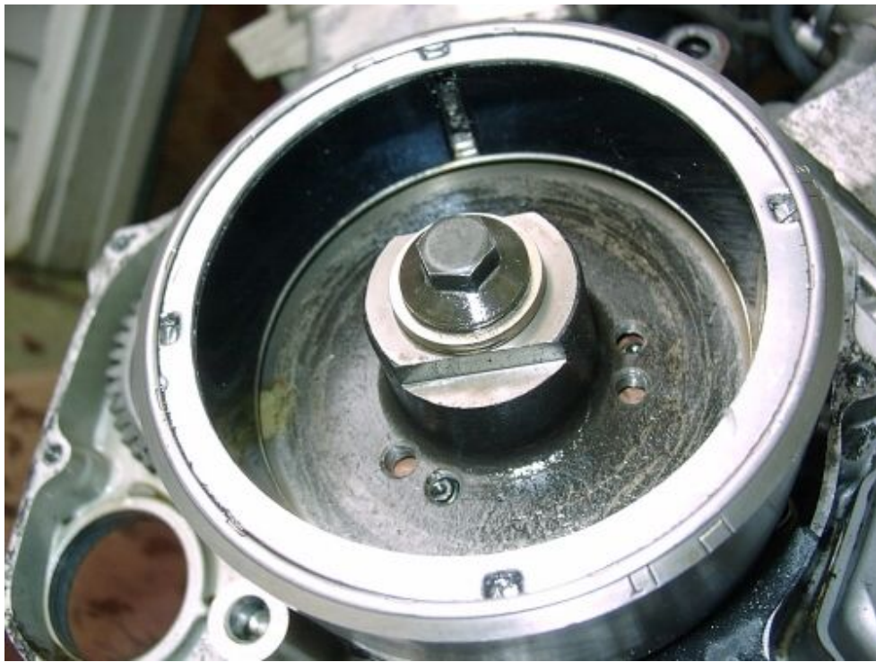
[Fig #2] : Two (2) Permanent Pole Magnets On Flywheel Rotor
